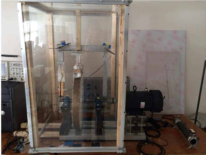
Figure 3 Maglev System with Safety Enclosure
